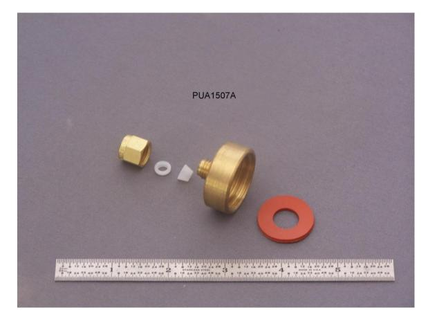
The Alcoa Bottle Adapter (25mm) provides the means to install a Sentry temperature probe into a bottle with a 25mm Alcoa closure for a test.
